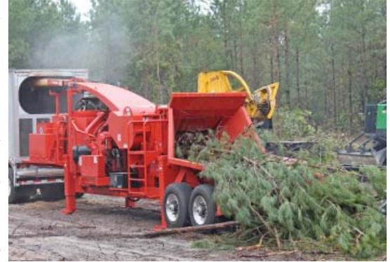
In-woods chippers use several different sources of energy to operate. Those sources are: electrical, pneumatic, mechanical, hydraulic, gravity, and thermal. It is very important that when the chipper is being worked on that all of these energy states are at zero. The chipper should be Locked and/or Tagged Out when it is being serviced, whether you are just changing a hose or changing the knives.
