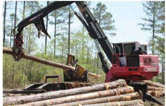
loader, you, the operator are in the direct line of fire. The fragments have been known to penetrate the Lexan side shields of loaders and still have enough force to fracture an operator’s jaw. When operating the processing head, when you grab a tree make sure the processor bar is not directly in line for you to see as you cut it. Process logs closer to the ground to reduce the distance chain shot fragments can travel.
