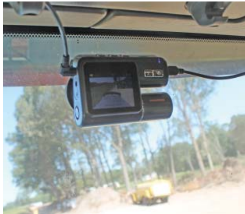
The dash mounted camera provides a wide bumper to bumper view of the front end of the truck.
